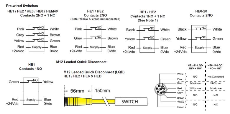
**CONTACT OPERATION -** The N/O contact(s) on Mechan safety switches are open when the actuator is away from the switch. When the actuator is within the specified operation distance, the N/O contact(s) will close and N/C contact will open.
