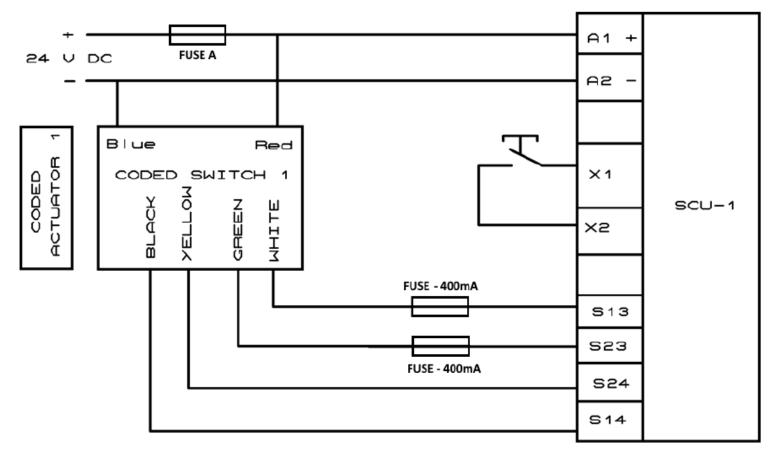
Fuse A: Main fuse for overall circuit including the contactors. 400mA Fuses: Fast acting (quick Blow) to protect all switch contacts.
