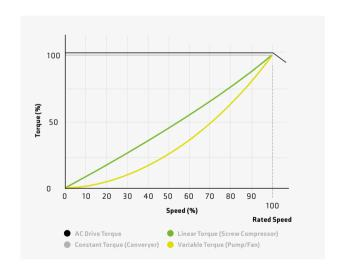
The most significant energy savings can be achieved in applications with a variable torque load. The cube law relationship between speed and power means that reducing a fan's speed in a variable torque load application by 20% can achieve energy savings of 50%. Therefore, for most motion control applications, reducing motor speed is often the easiest way to get large energy savings.
